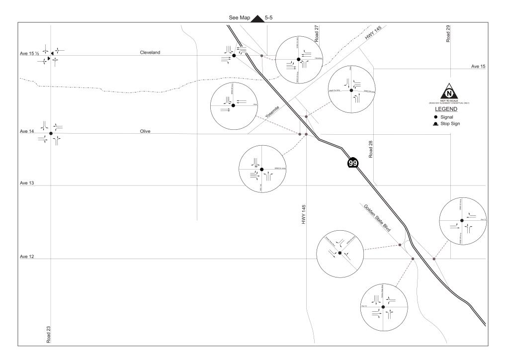
Figure 5-6 Madera Site – 2008 Lane Configuration and Intersection Control With Alternative C Mitigation
