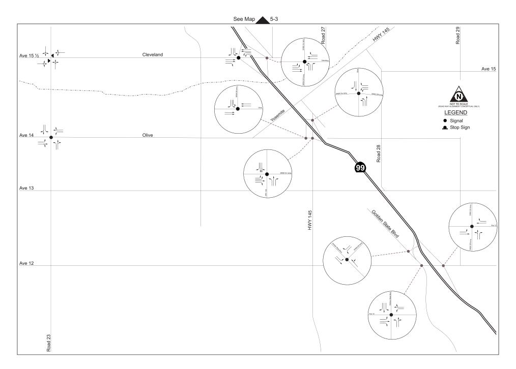
Figure 5-4 Madera Site – 2008 Lane Configuration and Intersection Control With Alternative B Mitigation
